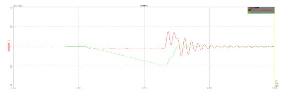
(2) Test once with the rated speed 0.50m/s, rated load 1250kg, system mass 4600kg.
